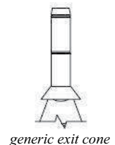
Figure 8 - Vertical Venting with a Metal Chimney System
